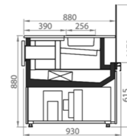
CUBE Pizza Slim with built-in unit L= 625, 1250, 1875, 2500 mm Display case can be equipped with a marble top
