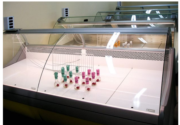
Experimental cabinet Ellipse CS with cross cooling system (Aisberg)
