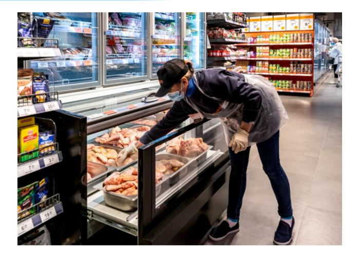
**The pull-out expositional surface** makes it easy to load products in boxes and containers. A good view of the products in the cabinet is achieved by the height of the display «windows» and the lighting in the upper and lower volumes.
